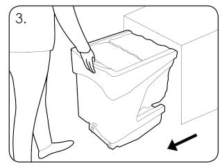
Using the integrated handle lip, wheel out the unit to deposit waste or to check how full the sacks are.
