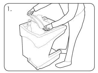
Lift up the sack retention and place the bag inside the caddy. Hook the bag over the sack retention band(s). Push the sack downwards back into position to secure the sack.
