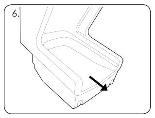
By tipping the unit slightly any liquids will flow out of the unit from the central spout The drip tray can be easily cleaned using hot soapy water once emptied.
