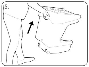
Use the recessed lifting handle to tip the unit to remove any spilled liquids collected in the drip tray.
