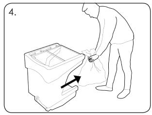
To remove the sacks, lift up the sack retention band and pull out the sacks from the rear of the unit, for safe manual handling.
